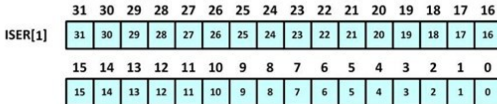
Figure 6-11: Set Enable Register (ISER[1]) for IRQ 32-63
