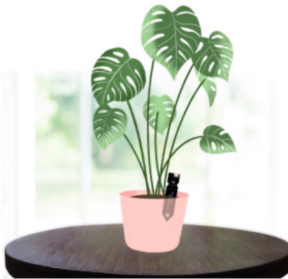
Figure 6.2 – How to place the moisture sensor
