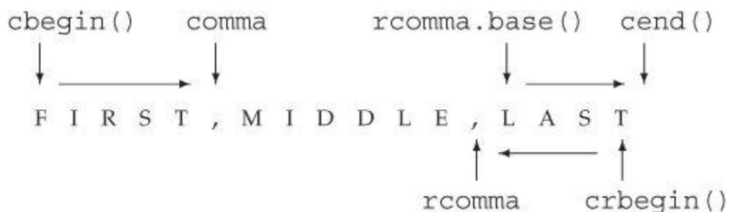
Figure 10.2. Relationship between Reverse and Ordinary Iterators
